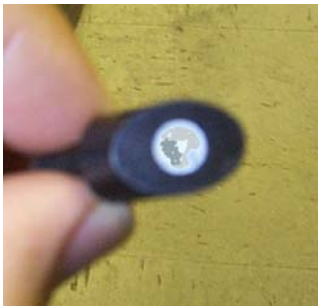
Missing retro (dead spot)
