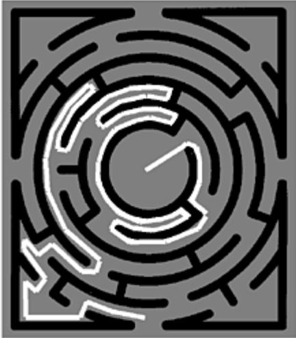
*Figure 1.2* Route through the maze using the left hand rule.
