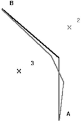
Figure 2.14 Sliver polygons as a result of digitizing the same line twice.
