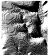
*Figure 9.11* Gridded DEM produced using inverse distance weighting on contour. contour, there is a rapid change in the interpolated heights, leading to a DEM which resembles a 'wedding cake'.
