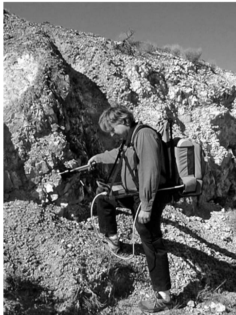
FIGURE 4.6. Field operator taking spectra of rock outcrop, using back-mounted spectrometer with fiber optic cable connected to probe. Photograph courtesy of Analytical Spectral Devices, Inc.
