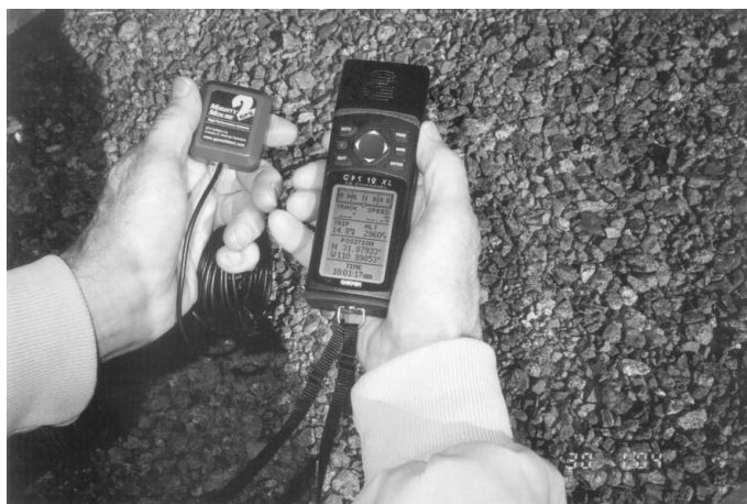
FIGURE 3.3. Hand-held GPS receiver suitable for field work with remote antenna attached. Photograph courtesy of Sue McCoy.
